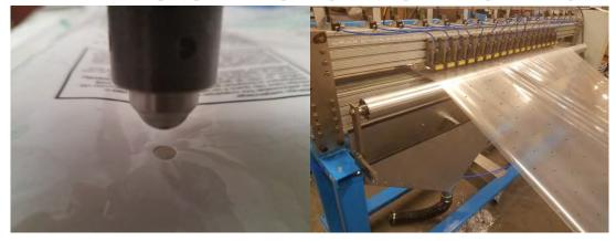
The Stewarts of America Electro-Pneumatic Punch Perforating unit is a field proven design. The machine has established itself in the flexible packaging industry as a preferred solution for consistent and reliable perforations in film, bags, paper and other products. Standard and optional functions let the machine efficiently produce round-hole patterns in a web that is in continuous or intermittent movement.
